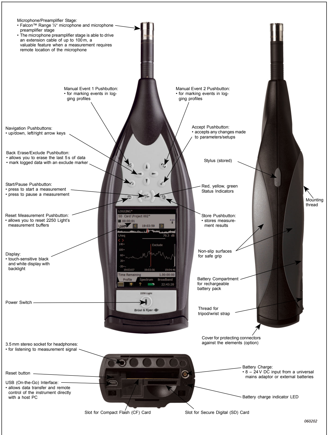
Fig. 1 Key features of 2250 Light
